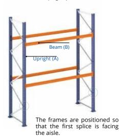
Position the remaining beams until all levels have been completed. To ensure that drill holes in the upright.
